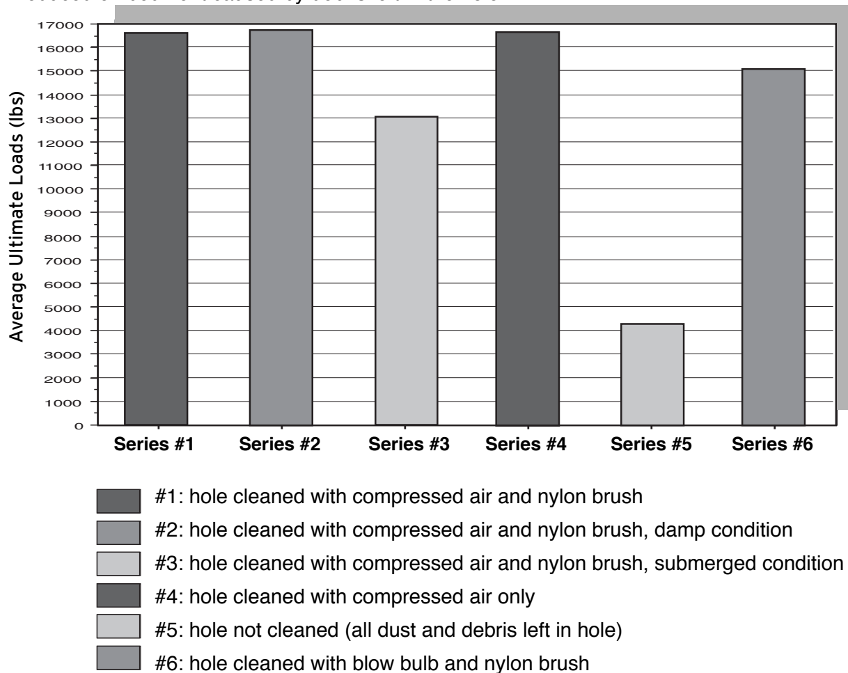
Fig. 5: Average ultimate loads of CIA-Gel anchors installed in holes left in various conditions
