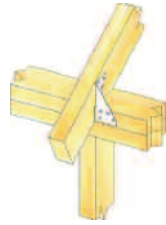
Typical RT4 truss/rafter to plate installation
