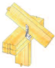
Typical RT15 truss/rafter to double plate installation
