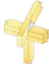
Typical RT6 truss/rafter to double plate installation
