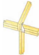
Typical RT5 truss/rafter to double plate installation
