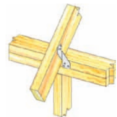
Typical RT12A truss/rafter to plate installation
