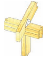
Typical RT6 truss/rafter to double plate installation
