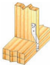
Typical RT8A stud to double plate installation
