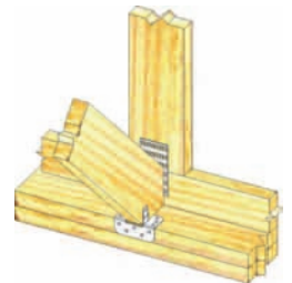
Typical HC520 gable brace installation
