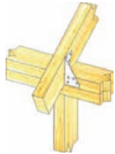
Typical RT4 truss/rafter to plate installation
