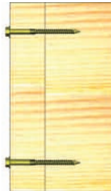
WS35 installed in (1) 13/4", (1) 31/2" Ply
